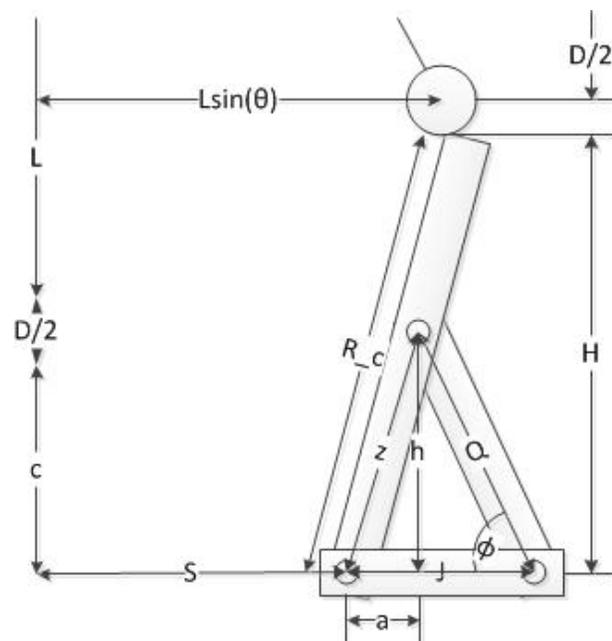
dimensions for the rotors and stators (the arm dimensions have already been calculated), all pendulums can be released at the same time.
